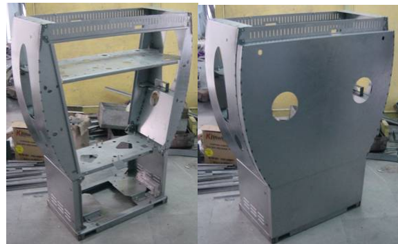
Figure 5. Gasoline dispenser prototype in process using CNC machining and bending
