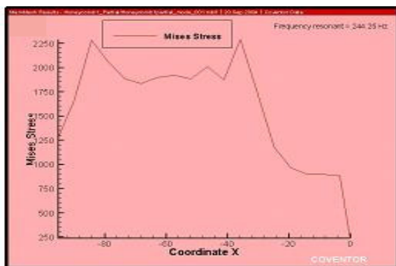
Figure 4b. Stress along longitudinal axis flexure length is plotted in Fig. 4(b) .
