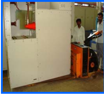
Fig.7 Structure handling with BOPT
